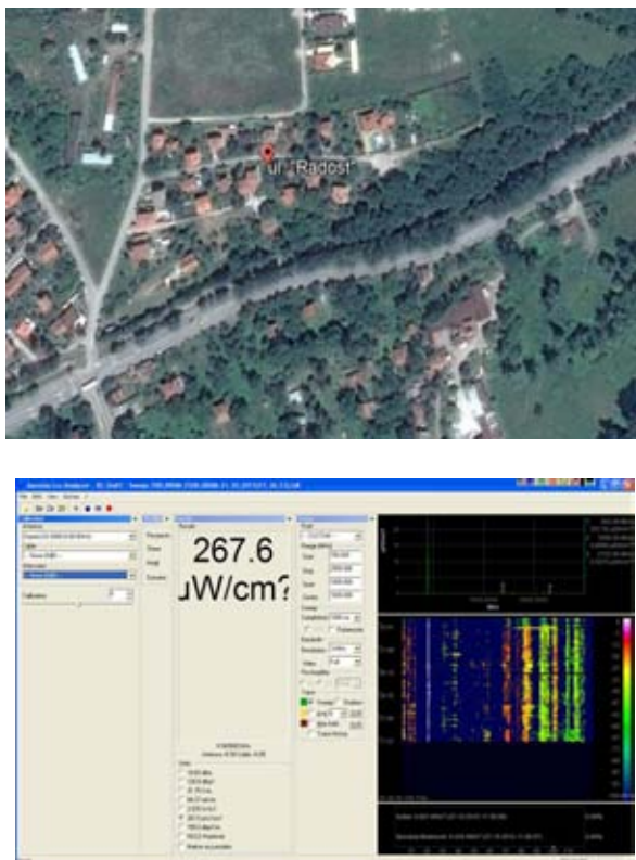
Fig. 1. Satellite photo of the territory of Bankya District, where the measurements of the density of EMR energy flow were carried out and the results of the measurements on a screenshot of the laptop to which the measurement device “SPECTRAN HF 6060” was connected
